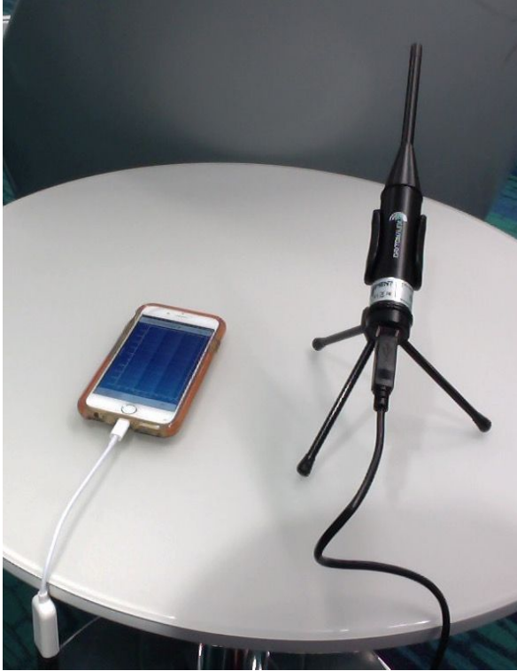
Figure 3: Experimental setup of microphone and Signal Scope App
