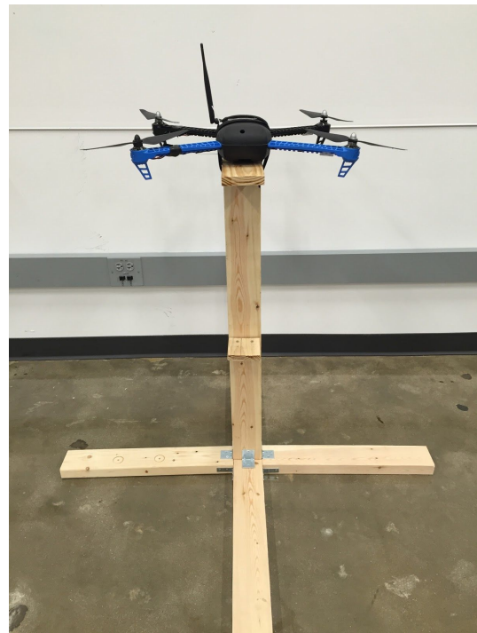
Figure 2: Test stand with IRIS + UAV securely strapped to it
